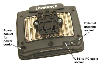
External connections on the back of the iWAY<sup>TM</sup> 600c.
